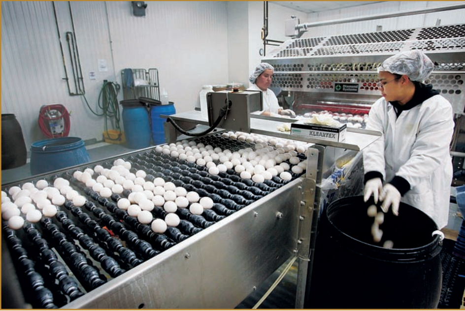
FIGURE 1.7 Juana Plascencia and Neomi Morrales sort and remove damaged eggs after they have been pasteurized at the National Pasteurized Eggs processing facility in 2006 in Lansing, Illinois. The pasteurization process destroys viruses, including avian influenza, and harmful bacteria, including Salmonella .
